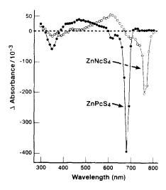
Fig. 3. Triplet-singlet difference spectra (10 nm resolution) of ZnPcS<sub>4</sub> and ZnNcS<sub>4</sub> as measured 1.2  $\mu$ s after flashing at 355 nm. The reaction mixtures were 10  $\mu$ M in sensitizer, 0.1 M in Na phosphate buffer of pH 7.4, 10 mM in cetylpyridinium chloride and 0.24 mM in oxygen (air saturated). The temperature was 25 °C.
