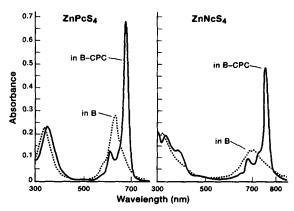
Fig. 2. Absorption spectra of 5  $\mu$ M ZnPcS<sub>4</sub> and ZnNcS<sub>4</sub> as measured in a 1.0 cm cuvette in 0.1 M Na phosphate buffer of pH 7.4 (B; dotted curves) and in B containing 10 mM cetylpyridinium chloride (B-CPC; full curves).
